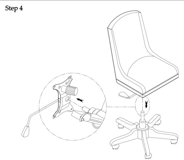
Note: To prevent possible damage to some type of flooring, never roll casters on unprotected hardwood or vinyl flooring. The lift mechanism is in a locked position for shipping. To unlock, pull straight out on the handle, and then the lift cylinder can be activated by lifting the handle.
